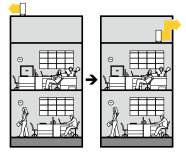
An external static pressure of 30Pa allows outdoor unit to be installed on balconies in high-rise building or spaces near louvers.
